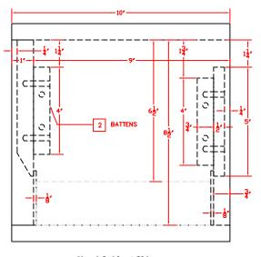
1/8" has been allowed for the front and rear faceplates. Generally, faceplates will not be that thick, so the result will be a small gap between the faceplate and the front, or rear face panels. If that bothers you, you will have to adjust the dimensions accordingly.
